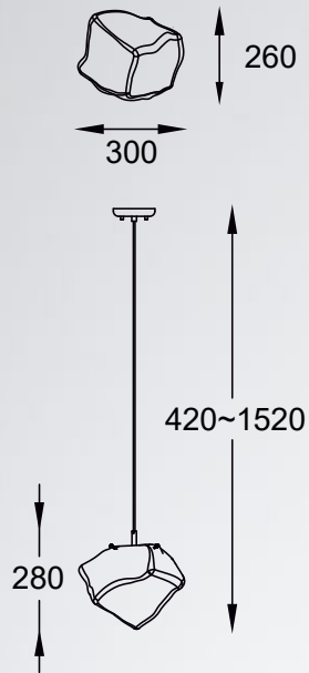
ROCK Pendant lamp P0488-01A-F4AC 1xE27 MAX 40W metal chrome body, crushed glass shade
